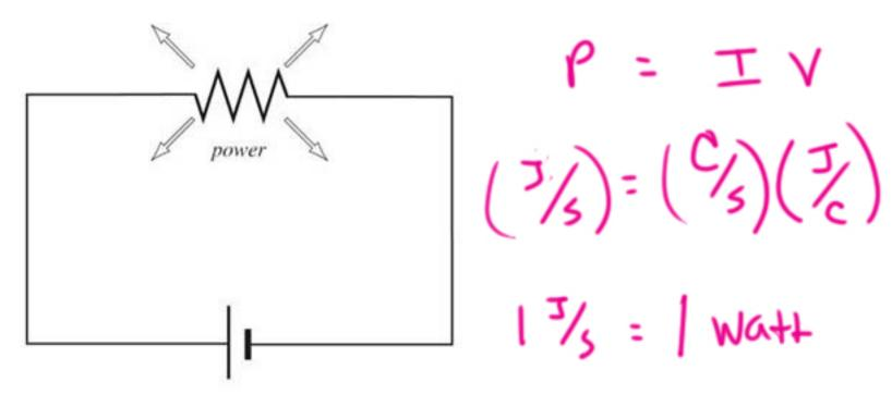
With neglible internal resistance, a battery delivers a steady voltage to a variable resistor. With  $P_i$  representing the initial power output, what is the final power of the circuit when the length of the variable resistor is halved?
