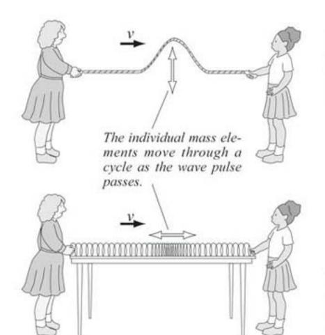
A transverse pulse. If the displacements associated with wave disturbances move in a direction perpendicular to wave motion, the wave is transverse.
