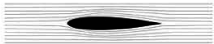
laminar (streamline) flow (low Reynolds number)
