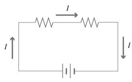
The positive terminal is the zone of positive potential in the circuit. This is where positive charges have high potential energy. It's good to visualize the charges 'falling' through the circuit from the positive to the negative terminal of the voltage source.
