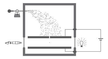
To determine the mass of a particular droplet, the experimenter observes the rate at which it falls in the earth's gravitational field. The drop reaches a terminal velocity, which depends on the mass of the droplet, the oil density and the viscosity of the air.
