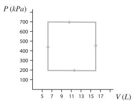
What is the difference between the heat taken en in by this engine and the heat that the engine expels each cycle?
