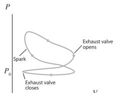
Under the cold air-standard assumption, the thermal efficiency,  $\eta_{th}$ , of the ideal Otto cycle is
