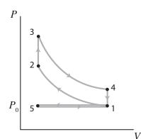
A detailed study of the performance of an actual gas power cycle is rather complex and accurate modeling of internal combustion engines normally involves computer simulation. The following diagram represents an actual internal combustion cycle. Notice that an actual cycle does not have the sharp transitions between the different processes of the ideal cycle.
