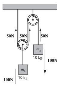
The tension in the rope is 50N to hold up the 10kg mass on the left. This translates as a net upward force of 50N on the mass on the right. Therefore, there is a net downward force of 50N on the 10kg mass. From Newton's 2nd Law,  $\mathbf{F} = \mathbf{ma}$ , we know then it is undergoing a 5 m/s<sup>2</sup> acceleration downward.
