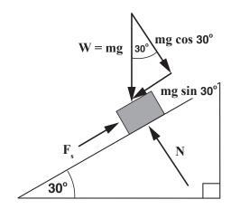
The threshold of static friction equals the product of the coefficient of static friction and the normal force. The static friction force which occurs will be less than or equal to this value.
