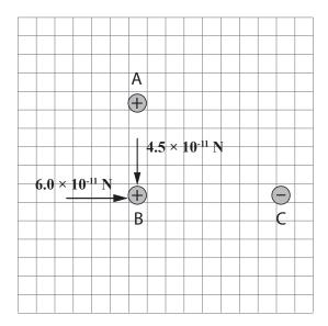
Now we perform vector addition to obtain the net force on B. The ratio of the forces are 3:4 and they are at a right angles, so vector addition will conform to the simple 3:4:5 right triangle ratio. A clue was provided in that the electric field strengths in the question stem have scientific notation coefficients 3 and 4.
