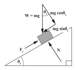
Here it is afterwards. (Note that static friction force has been replaced with kinetic friction force.)
