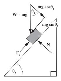
The normal force, **N**, must be equal and opposite to the component of the block's weight perpendicular to the plane. As the angle of incline is increased, the component of the weight perpendicular to the plane decreases and so does the normal force.
