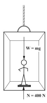
Above is a free body diagram corresponding for the man on the elevator. We can derive an expression for the net force on the man from this free body diagram and use Newton's 2nd Law to relate this net force
