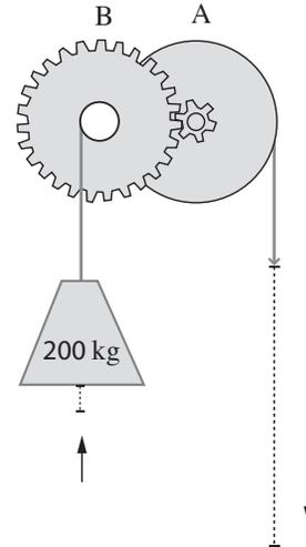
Let's feel our way with conversion factors. We know that one tooth of gear B moves forward after contacting one tooth of gear A, so we can use this to determine the ratio of revolutions of gear B to gear A.
