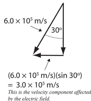
As with projectile motion, to answer the question of time in flight, we first need to ask how long it takes the electron to reach the peak. The time in flight will be twice that value.
