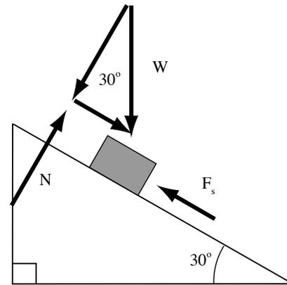
For sliding to happen a force of half the weight must be able to overcome the force of static friction. The maximum value of the force of static friction is equal to the product of  $\mu_s$  (the coefficient of static friction) and the normal force, which equals in magnitude the component of the block's weight perpendicular to the plane. This perpendicular component is equal to the product of  $\cos 30^\circ$  and the weight. In other words, the following is the condition of sliding:
