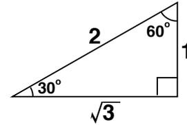
So the component of the weight parallel to the plane equals the product of  $\sin 30^\circ$  and the weight, and the component of the weight perpendicular to the plane equals the product of  $\cos 30^\circ$  and the weight.  $mg \cos 30^\circ$  also equals the normal force.
